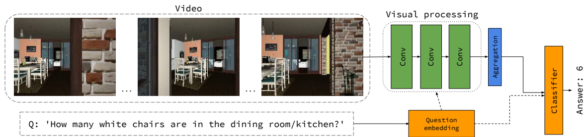
Figure 3.1: High-level description of the VideoNavQA task and our approach. Each example received by the ML system contains a video of a trajectory inside a house and a question about the visual stream. The system processes this multimodal input to produce an answer. We tackle the task via already-established VQA paradigms—where the language signal is used to condition the visual processing—and build extensions of these methods that account for the temporal dimension of the visual input.
